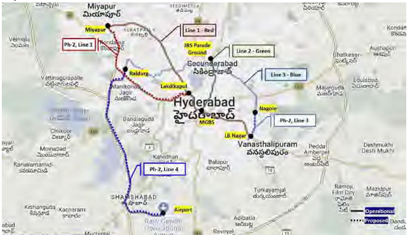
Figure 4-2: Airport Metro Proposed Alignment (Phase-2 Line 4)
