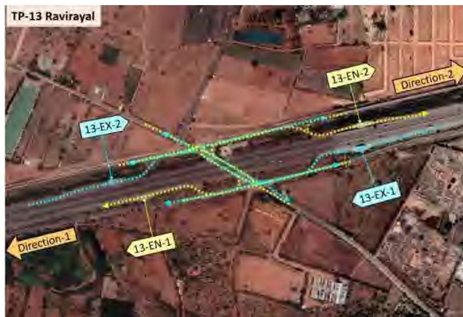
Figure 1-7 : Diamond Type Interchange with 4 toll booths
